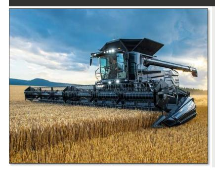
Smart combines improve the ability of the operator to automate adjustments usually made by skilled operators. A typical smart combine uses cameras and sensors to detect changes in crop conditions so combine adjustments can be made automatically and maintain optimal performance. **Five key environmental benefits** were identified to be quantified as a result of P.A. technology adoption
