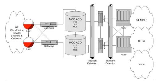
BT MCC (Multimedia Contact Centre) is a network-based, multimedia IP ACD. The MCC Platform can seamlessly handle both inbound and outbound TDM calls, VoIP and Video streams, collaboration, email, and chat. To facilitate the various interaction methods, the MCC platform is tightly interconnected with BT's voice and IP networks to provide a seamless and a very flexible interaction routing matrix.
