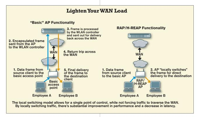
Edge Access Points, or H-REAP, that extends central WLAN management to remote sites. Both the controller appliance and remote AP options provide WLAN deployment consistency, direct remote troubleshooting capabilities, wireless intrusion prevention system (WIPS) capabilities to enhance RF visibility, and the knowledge that approved corporate WLAN security standards are being extended to all locations within the organization.
