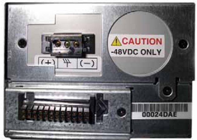
RACKABLE'S DUAL BLIND-MATING CONNECTORS PROVIDE CONNECTIVITY FOR ETHERNET, SERIAL AND POWER.
