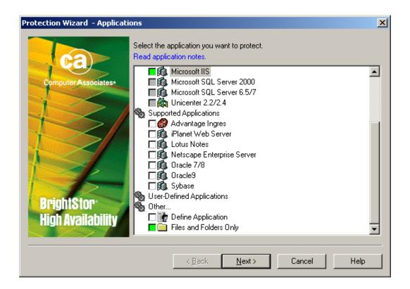
After installation, the system administrator configured BrightStor High Availability by creating a protection task using the Protection Wizard which is part of the BrightStor High Availability Manager program. The protection task defines the primary and secondary servers, the failover criteria, various replication settings and one or more workloads (the parts of the primary file system that are to be replicated to the secondary).
