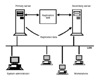
The diagram above shows a simple BrightStor High Availability installation in which a secondary server is protecting a single primary server, with a single LAN connecting the two and hosting a number of client workstations.
