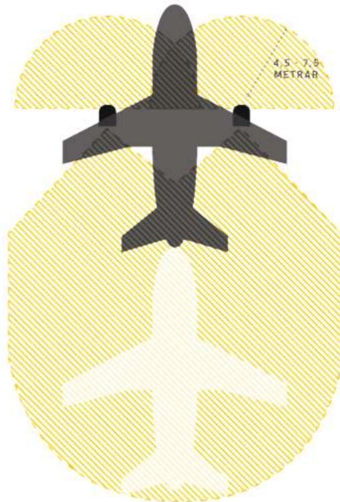
Danger from jet engines due to suction and jet blast
